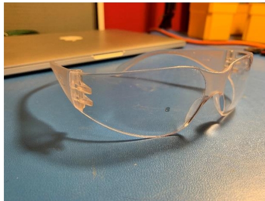
Figure 13: Example of eyeglass protection from solder spit
